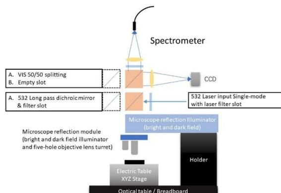
Single Channel model with 532nm exciting laser for Raman microscopy application
