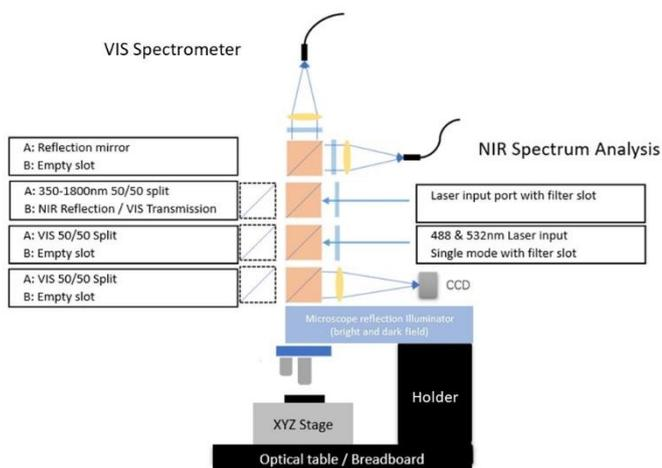
4 Channels setup with VIS to NIR Spectrometer, High resolution camera, and Multi wavelength excitation laser
